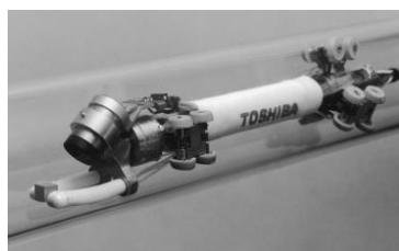
Fig. 9 Micro inspection robot carrying a recovered object in pipe [13].
